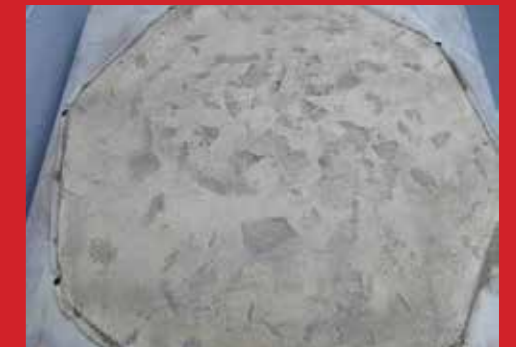
Fosroc Matacryl RB passed test, which involves 2M cycles of abrasion from ballast directly on top of the membrane
