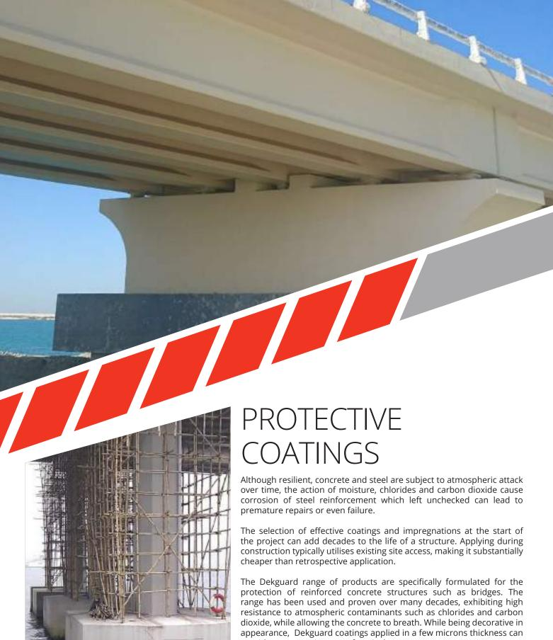
provide many centimetres of equivalent concrete cover.
