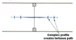
Supercast range incorporates both of these principles. The products offer a fully continuous 4 bulbed design maintaining both valve & tortuous path principles. These principles are maintained in the transition from Rearguard profiles in floors to centrally placed profiles in walls.
